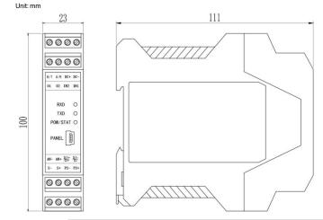
1.3 Installation methods 35mm rail installation
